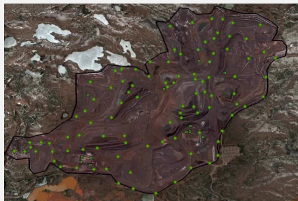
Wi-Fi mesh network in open pit mine with ~100 APs covering an area of 2 km 2 , or roughly 80 m cell range. It is possible to cover the entire area with 1 LTE site!
